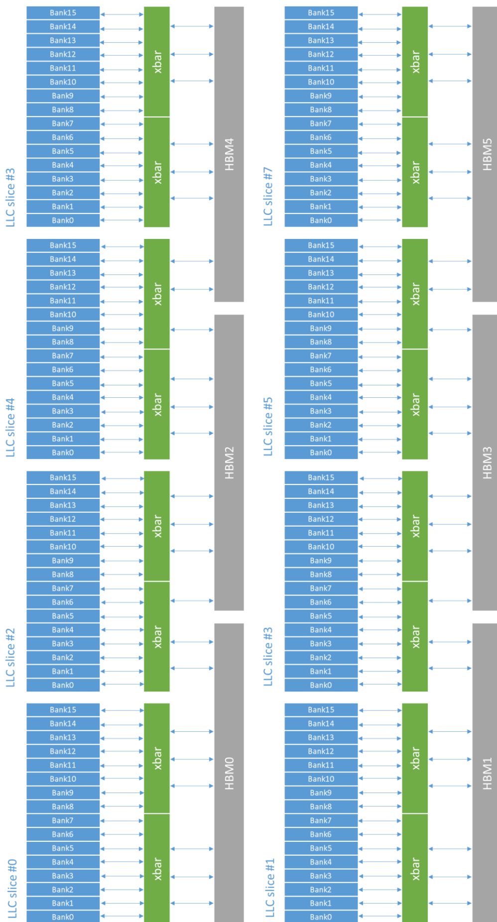
Figure 9-6 Aurora VE connection between LLCs and HBMs
